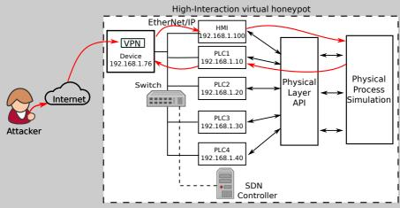
Attack propagates over the simulated components
