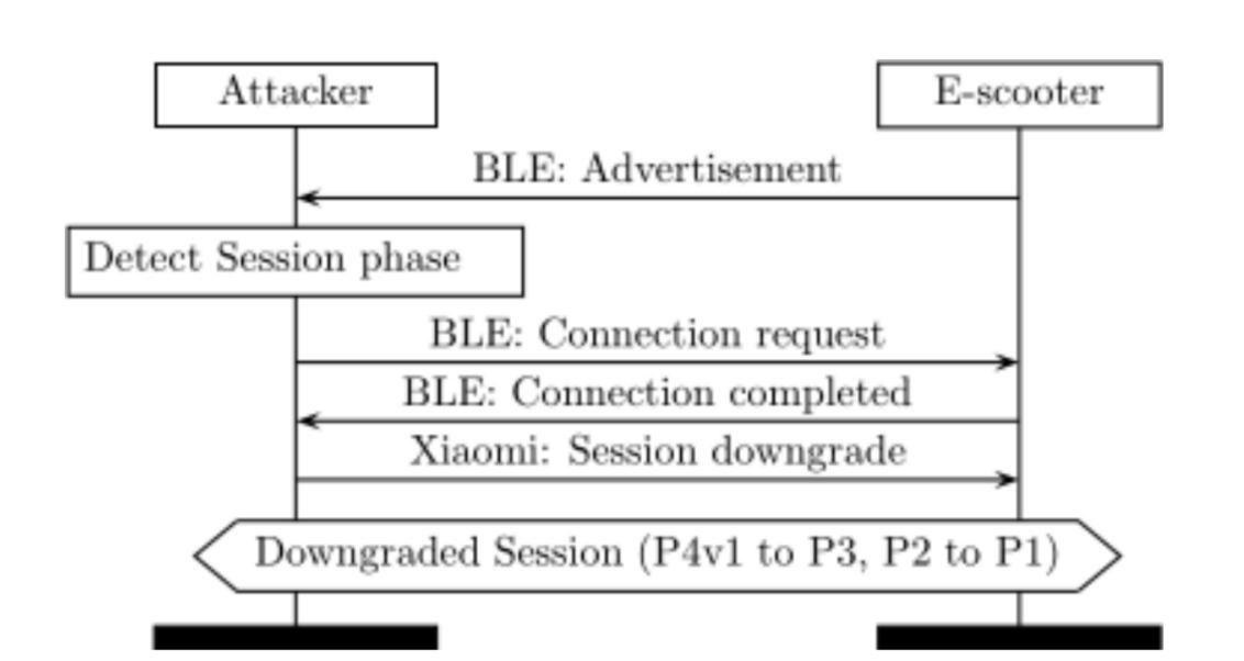
The attacker sends an unprotected Session downgrade command, downgrading P4v1 to P3 or P2 to P1.
