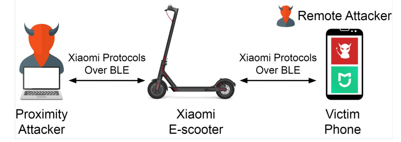
The e-scooter is paired with the user, software-locked, and password-protected. The attacker sends BLE packets from proximity, or installs a malicious Android app on the phone of the victim. She knows Xiaomi Pairing and Session phase protocols. She does not need physical access.
