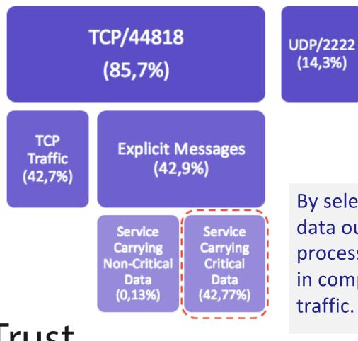
By selecting CIP services with critical data our proposal avoids additional processing and bandwidth overheads in comparison with signing all CIP traffic.
