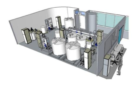
Secure Water Treatment (SWaT) is a testbed for research in the area of cyber security.
