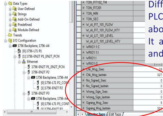
Different tags were configured at PLC program to store statistics about signing/verification process. It allows to monitor the process and debug it.
